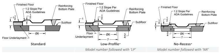
\*For Low-Profile and No-Recess models, a 7" x 18" x 3/4" blockout centered with the drain is required
