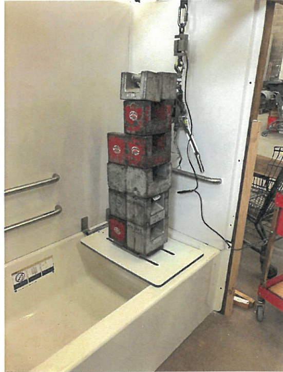
Photo 10 – Load test of 523lbs on seat
