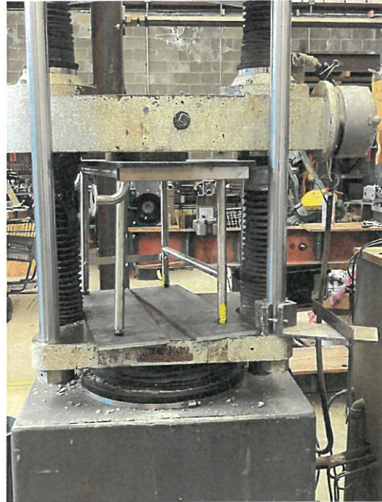
Photo 14 – Seat load test in hydraulic apparatus
