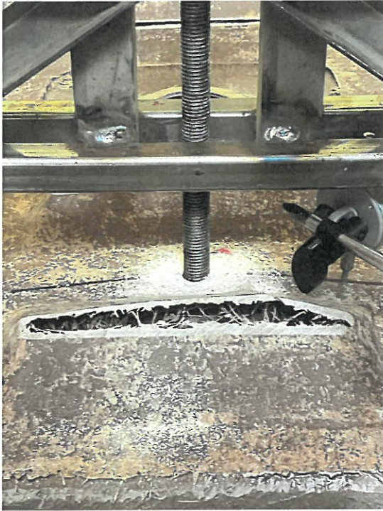
Photo 13 – Off-center load test failure location
