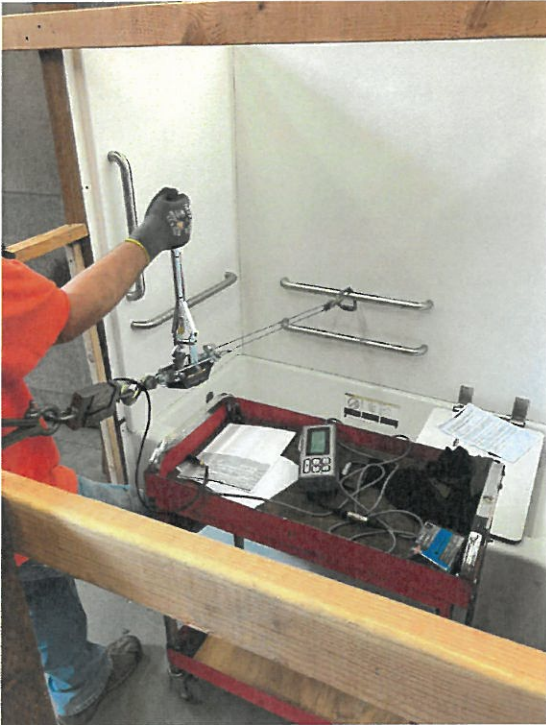
Photo 7 - Horizontal Test at Location E
