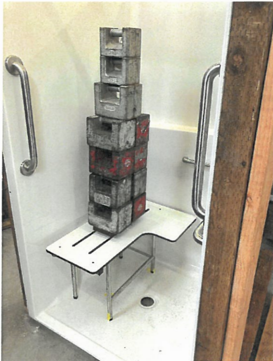
Photo 3 – Seat Load Test of 523lbs
