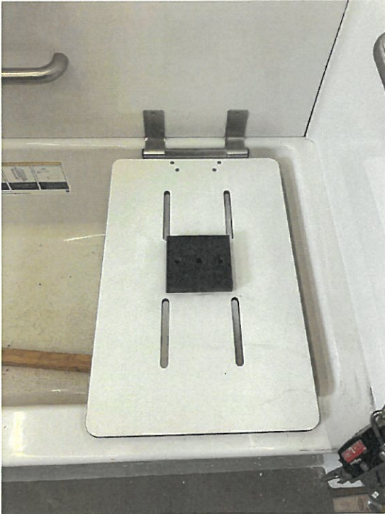
Photo 9 – 5” x 5” bearing plate for seat load test
