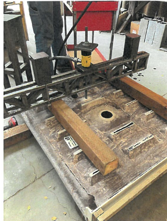
Photo 12 – Off-center load test of floor pan
